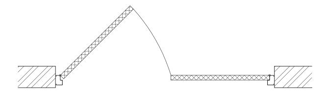
STEEL-TEC DOUBLE LEAF FIRE EXIT DOOR OUTWARD OPENING - LH ACTIVE
