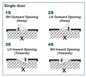
To help determine where your hardware is to be positioned on the door, view the door from the hinge side
