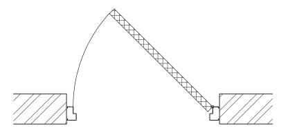
STEEL-TEC SINGLE LEAF FIRE EXIT DOOR OUTWARD OPENING - RH HINGED
