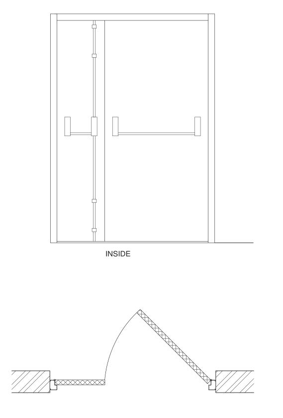
STEEL-TEC LEAF & HALF FIRE EXIT DOOR OUTWARD OPENING - RH ACTIVE
