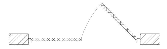
STEEL-TEC DOUBLE LEAF FIRE EXIT DOOR OUTWARD OPENING - RH ACTIVE
